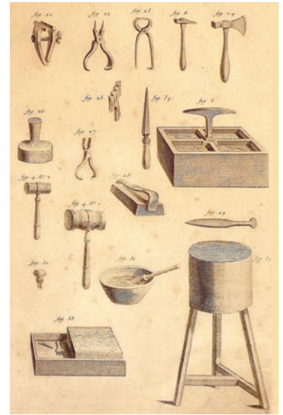
2 This print shows the tools used for brass work by a lamp-maker (ceinturier) from 1740
