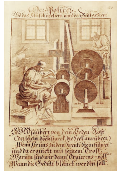
3 Print Der Polierer (metal polisher), known in Vienna as a Metall-Schleifer, they worked on copper-based metals. The large wheel is used for the rough polishing, the small one is a wheel of textile rags for the final polishing
